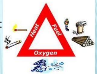
Basically, three elements are needed for a fire to start: A source of fuel; a source of heat; and Air (Oxygen). These three factors have been diagramed as the three sites of a triangle.
