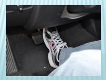
Now that you have begun to apply the brake, it takes some time and distance before the vehicle actually comes to a complete stop. This is called "Braking Distance".
